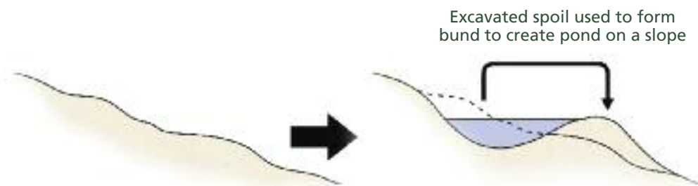
Figure 5. Spoil can be used to form lower bank of pond on slope.
